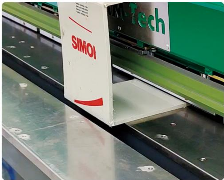
0 - 95° Bending by one sheet
