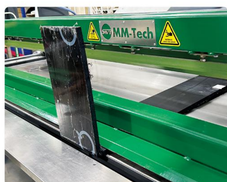
0 - 95° Bending by one sheet
