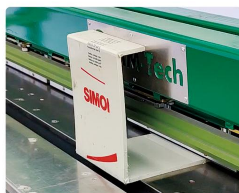
0 - 95° Bending by one sheet
