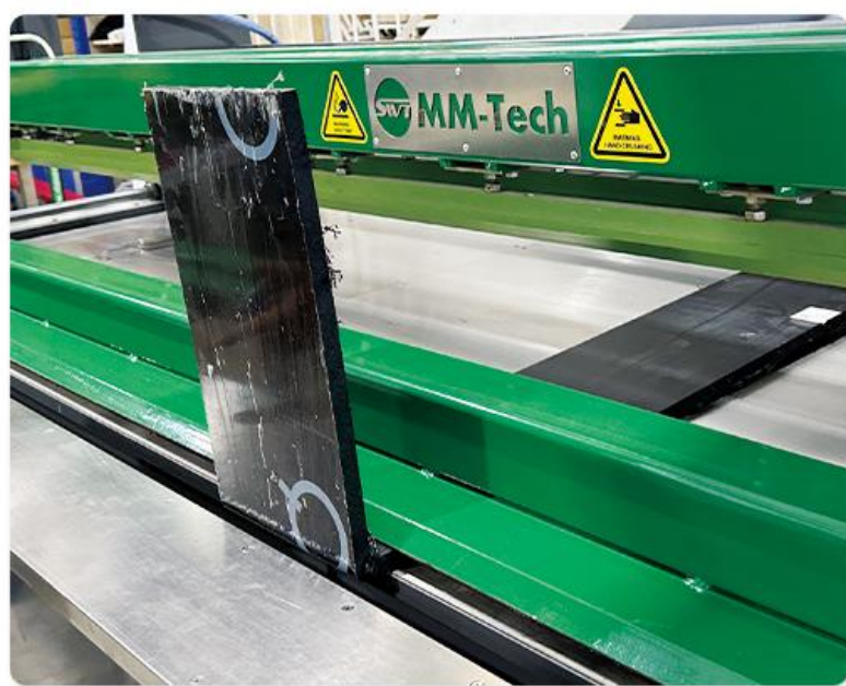
0 - 95° Bending by one sheet
